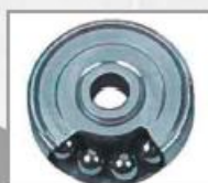
Autobalancer The autobalancer consists of steel balls, lubricated in oil, that freely move around the drive shaft in a housing similar to that for ball bearings, and so perfectly level out any imbalance.
